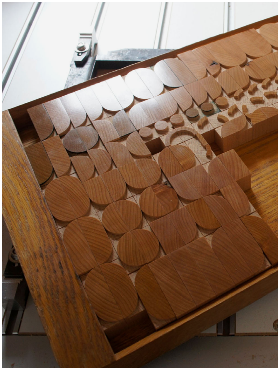
Figure 8. LetterIsland, Typemods , remaking: a modular typographic system inspired by Spanish typefaces from the 1930s, manufactured using a CNC milling machine (Matthias Beck).
